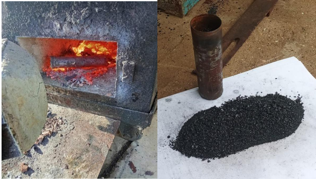
Figure 2. The Process of Conductive Charcoal Formation
